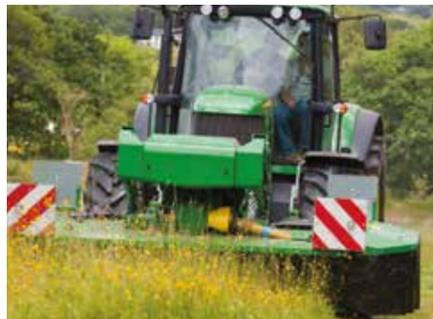
**EN:** Rotary mowers are equipped with protection cloths to protect the surrounding areas from thrown objects. An especially strong textile, developed by SATTLER PRO-TEX, fulfils the criteria of relevant norms ISO 17103 and EN 745 to comply with relevant safety standards.
